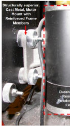
Note the engineered aluminum mounting brackets under a Brent wheel (silver) as opposed to bent, thin metal supports in other wheels. Also noticed the tough powder coat paint (black). Black powder coat is paint that is actually baked onto the surface, making a very durable protective coating.
